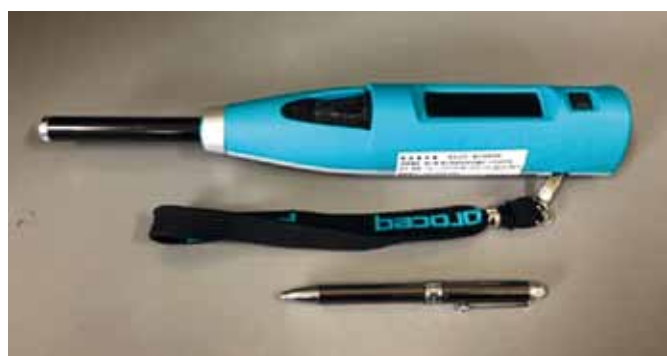
Fig. 8 – Silver Schmidt hammer (photo: Sakane).
