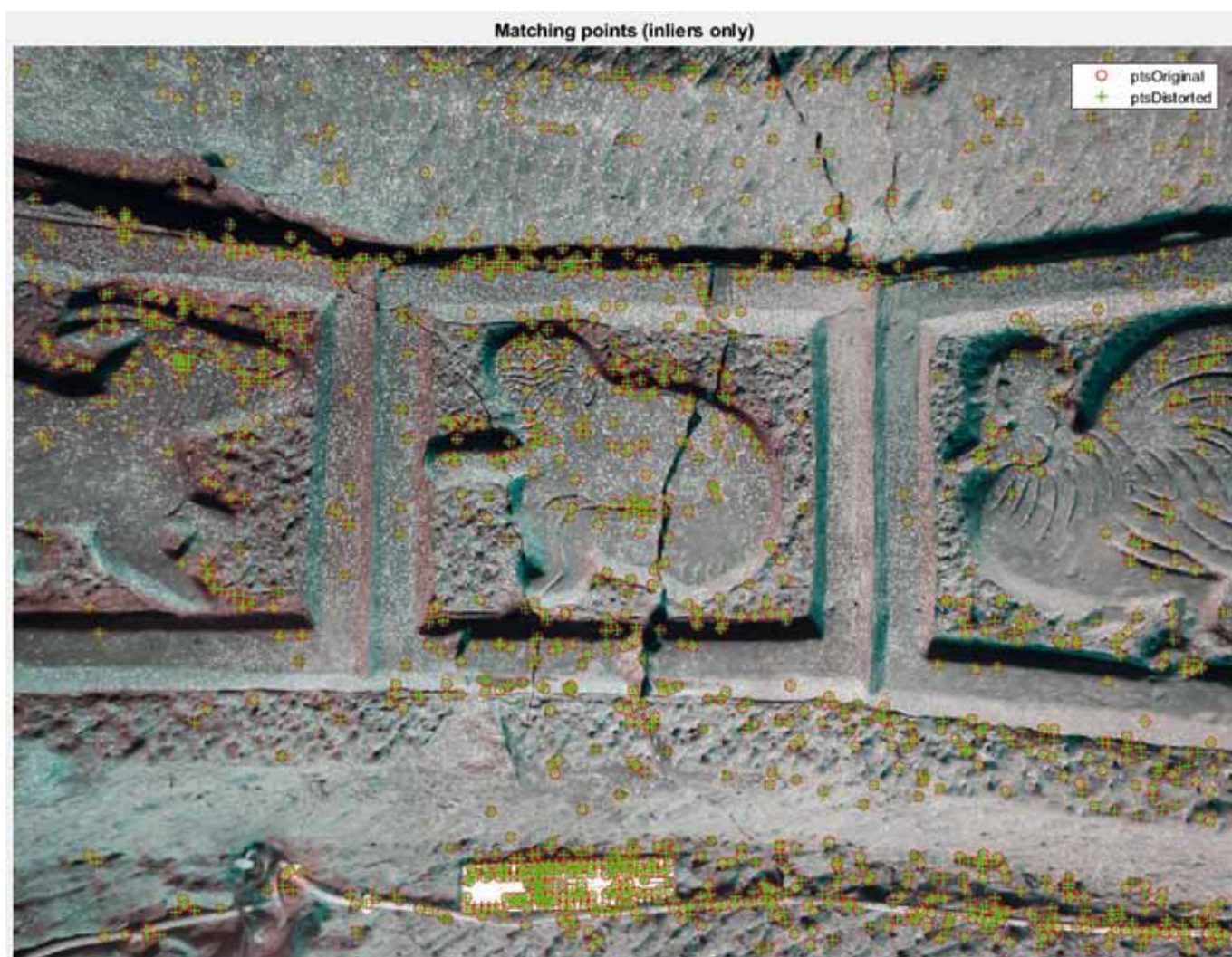
Fig. 9 – Result of two image matching. No differences have been found: as you can see detected feature points overlap (photo: ISASI/CNR©).
