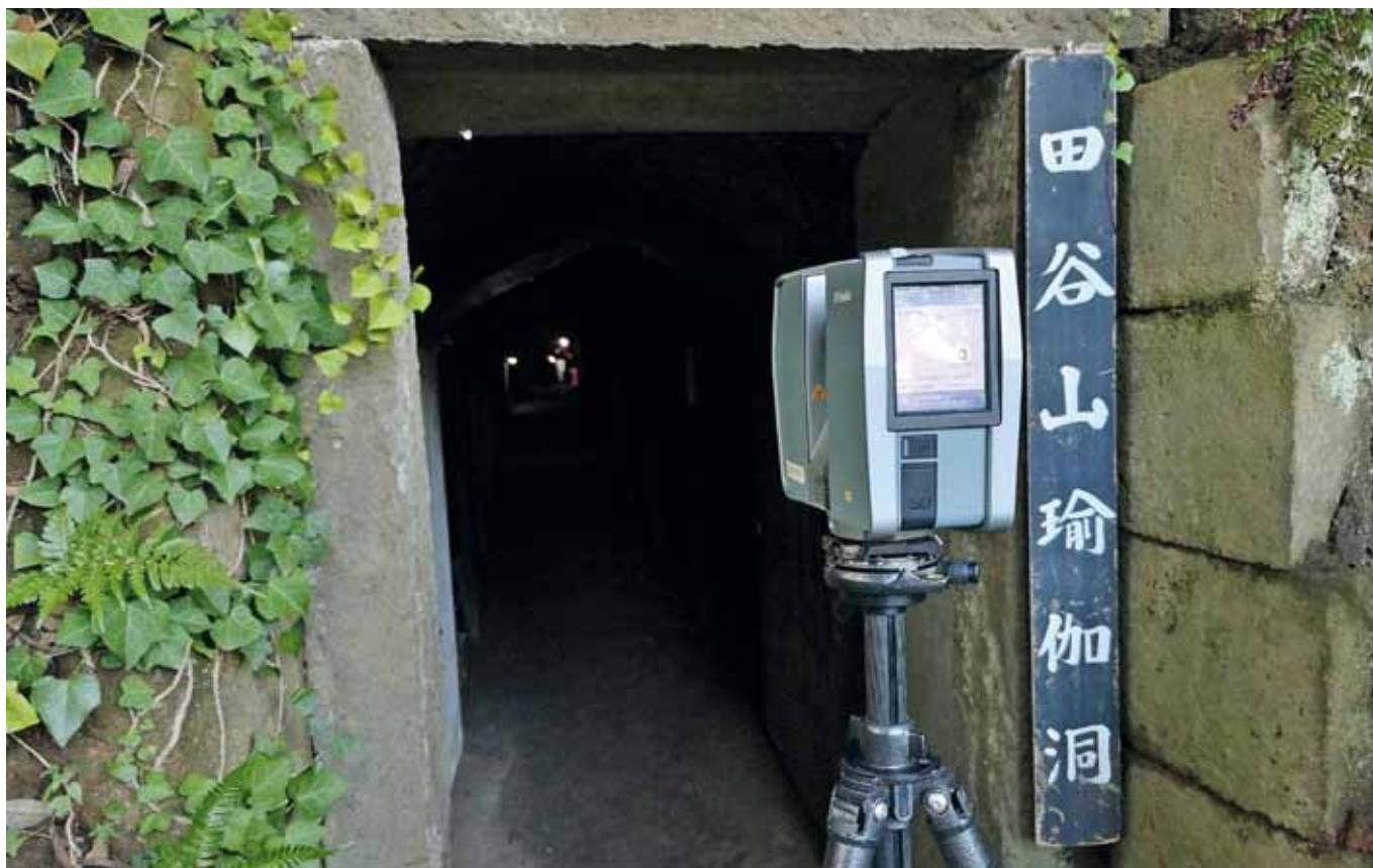
Fig. 2 – Entrance of Taya Cave and the terrestrial laser scanner used for the topographic measurement, Trimble TX5 (photo: Y. S. Hayakawa).
