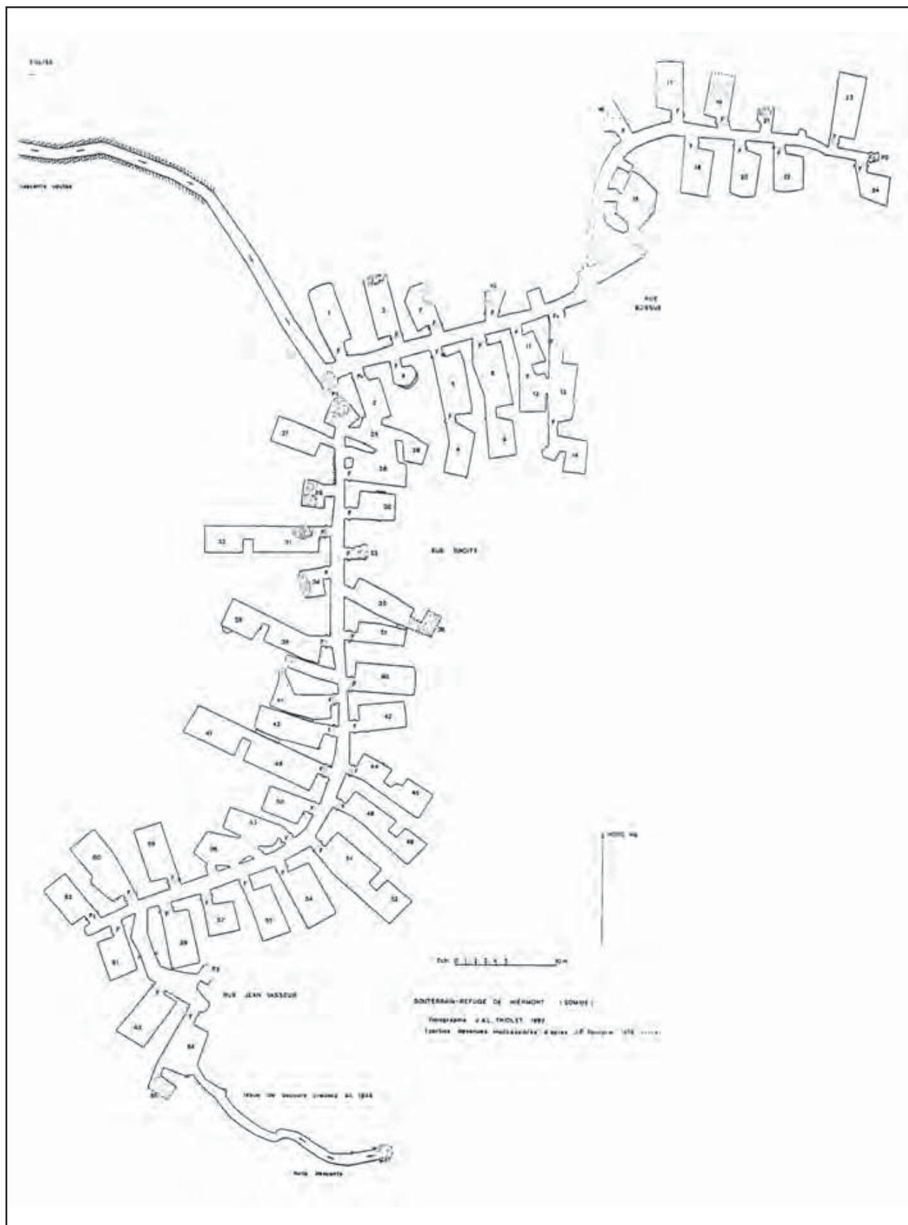
Fig. 11 - Plan of the village underground refuge of Hiermont, region of Amiens, France (topography J. & L. Triolet 1992 and after J.-P. Fourdrin 1976 for inaccessible parts).
