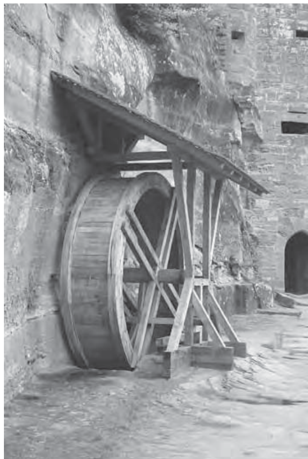
Fig. 17 - Dahn: treadwheel of a hoist recreated.
