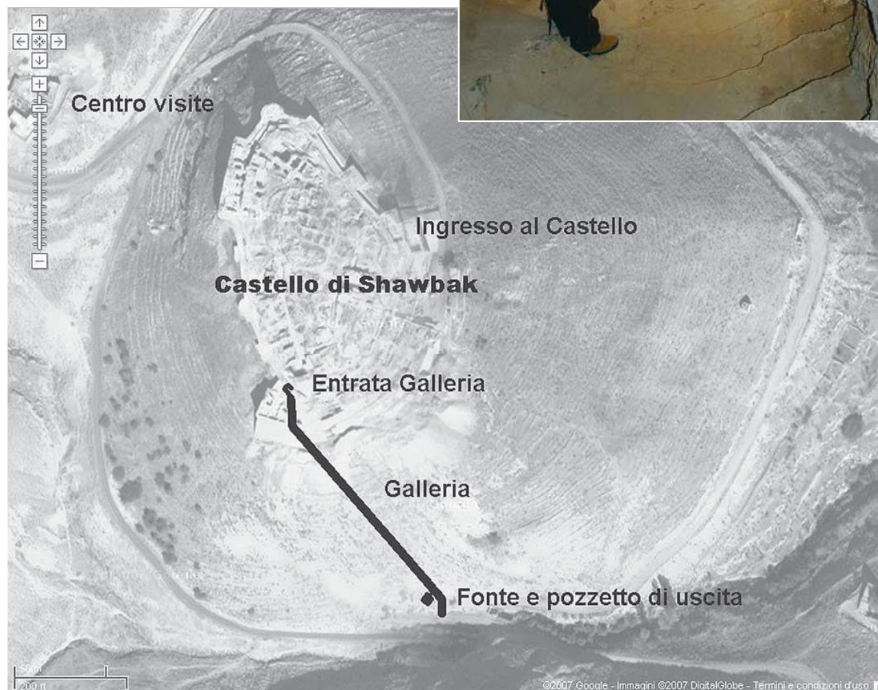
Fig. 7 - Bird's-eye view of the Shawbak Castle area, indicating the Ain al Ragaye spring diversion tunnel (drawing C. Germani).
