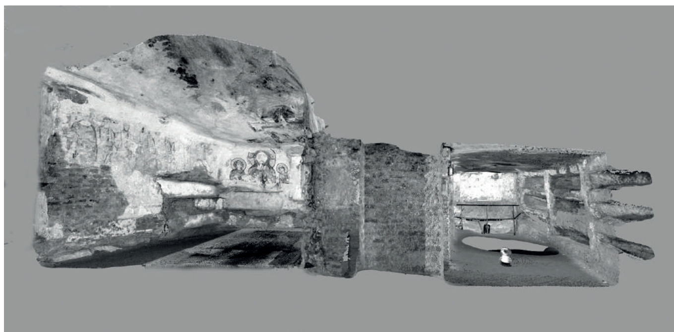
Fig. 4 – Perspective view after the points cloud of a lateral room with wall paintings (image by M. Carpiceci).
