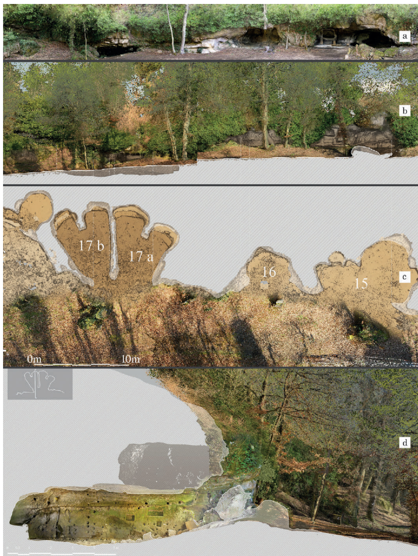
Fig. 8 – a) Prospectus in SFM, processed with Metashape Pro. A.A. 2021/22 (graphics S. Leone, D. Santini, E. Vergari); b), c) survey with Riegel, and zf. The colour data are integrated with those in black and white, treated with different pigmentation. A.A. 2019/20 (graphics B. J. Snickars); d) environmental section, integrating Riegel data with SFM processing in Metashape Pro. A.A. 2019/20 (graphics B. J. Snickars).
