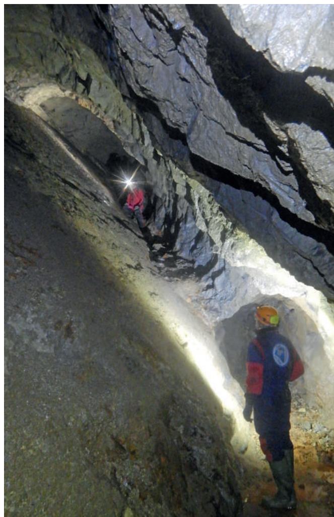
Fig. 5a – Mud mine: the underground works along the main quartz vein (photo Paolo Testa).
