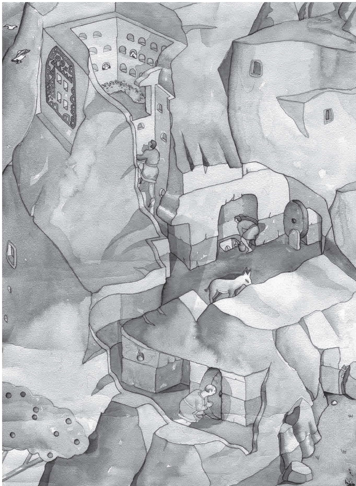
Fig. 8 – Rendering of a Cappadocian underground shelter with an internal entrance for people to a dovecote that could also be used as a last refuge in the case of raids. In the Mimar Sinan shelter (Kayseri), and Mucur (Kırşehir), the flight windows for pigeons open into the ceiling (chimney) instead of in the vertical wall (drawing R. Bixio).
