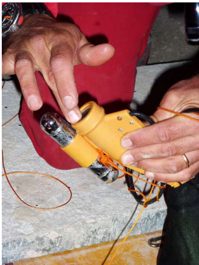
Fig. 11: a well camera that is to be integrated with a light source. Alternately, if size allows, a protected camera endowed with lights can be used (photo Mario Mazzoli).
