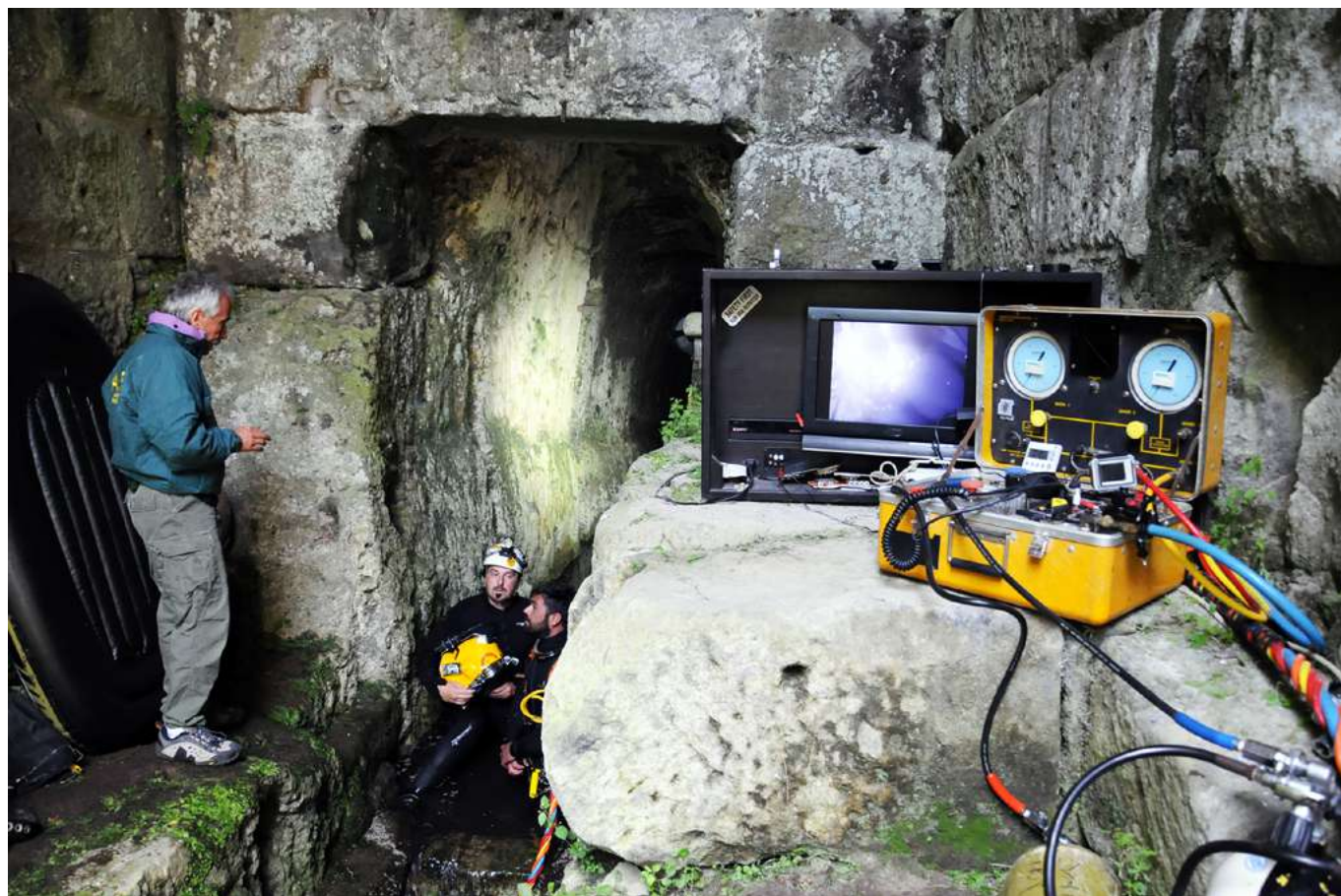
Fig. 6: workstation that fuels, detects and controls the breathing mixture and the audio and video signals (photo Marco Vitelli).
