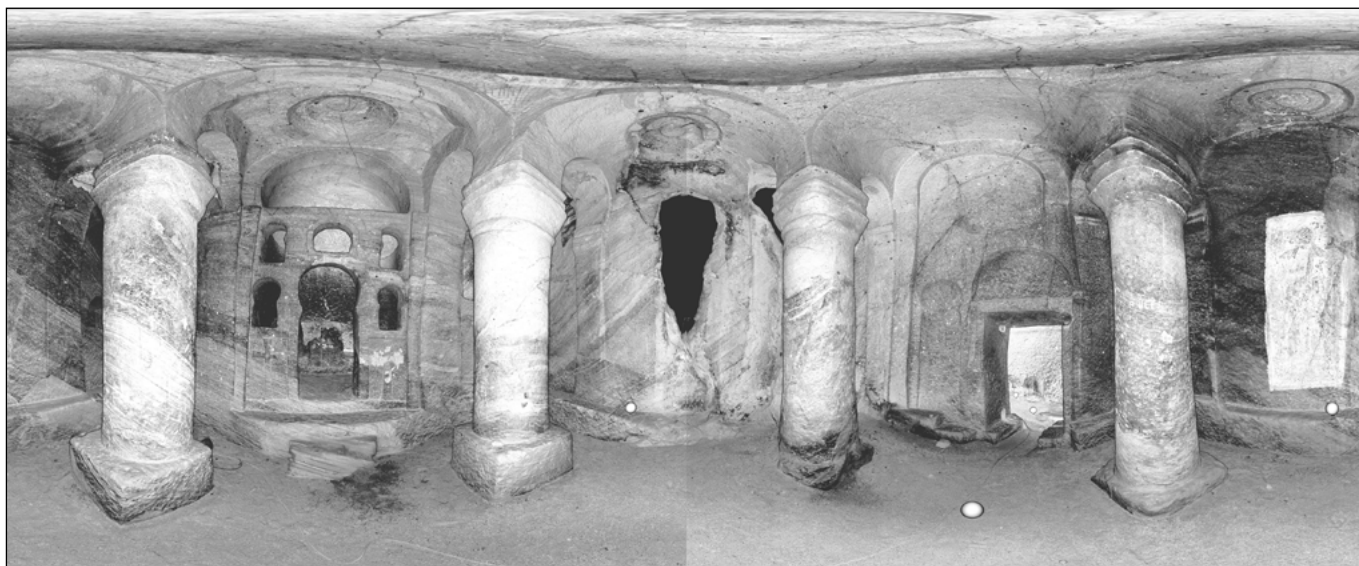
Fig. 3: the panoramic view represents the 2D editable point clouds. Due to the geometry of the image it is possible to modify accurately the central band and not the marginal part (image by A. Angelini).
