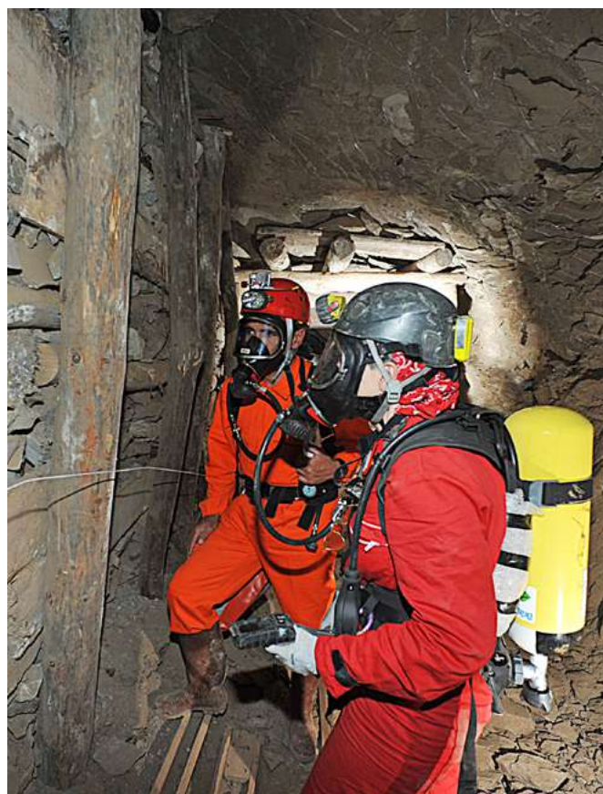
Fig. 2: speleologists with breathing apparatus and gas detector.
