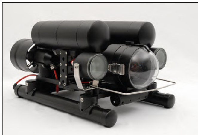
Fig. 14: underwater ROV produced for our survey (photo Engin Aygün).
