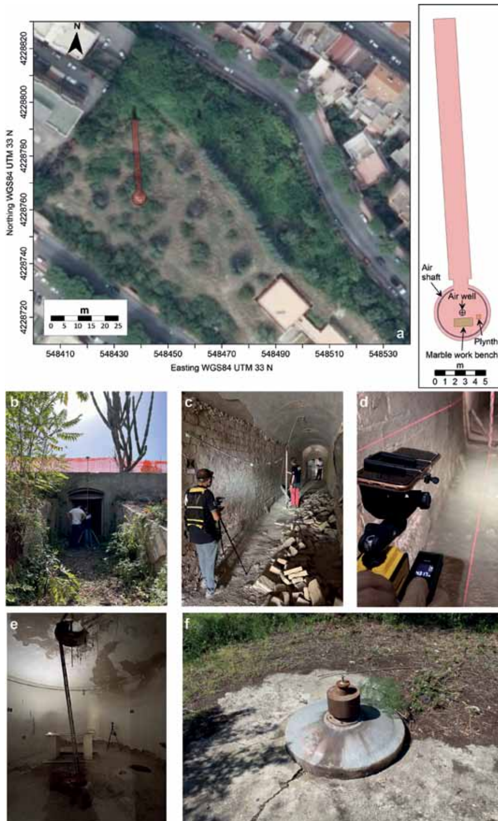
Fig. 1 – From the top to the bottom, and from left to right: a location of the gallery and its planimetry (background image from Google Earth); b entrance of the gallery; c internal view of the gallery during topographic survey operations; d particular of the topographic survey system; e the final circular room, aimed to host geophysical instrumentation; f the cupole of the final room outcropping from the ground ( draft by M. Cangemi ).
